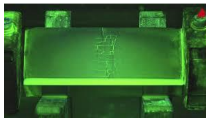
Gambar 3. Hasil Magnetic Particle Test (Sumber: Dokumen PT. Cipta Mulia Kreasindo)
